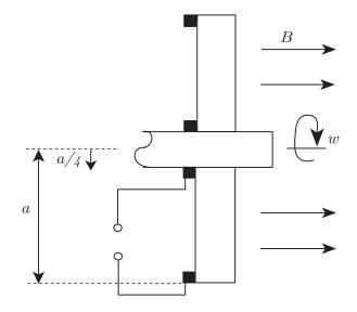
**3.2.** A homopolar generator consists of a metal disc of radius a and a central axle which has radius a/4. The disc has resistivity  $\rho$  and thickness t. It is rotated in a uniform magnetic field B about an axis through the centre, which is parallel to B and perpendicular to the plane containing the disc, at an angular frequency  $\omega$ . Thin ring brushes make good electrical contact with the disc near the axle and near the outer rim of the disc as shown.
