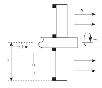
A homopolar generator consists of a metal disc of radius a and a central axle which has radius a/4. The disc has resistivity  $\rho$  and thickness t. It is rotated in a uniform magnetic field B about an axis through the centre, which is parallel to B and perpendicular to the plane containing the disc, at an angular frequency  $\omega$ . Thin ring brushes make good electrical contact with the disc near the axle and near the outer rim of the disc as shown.
