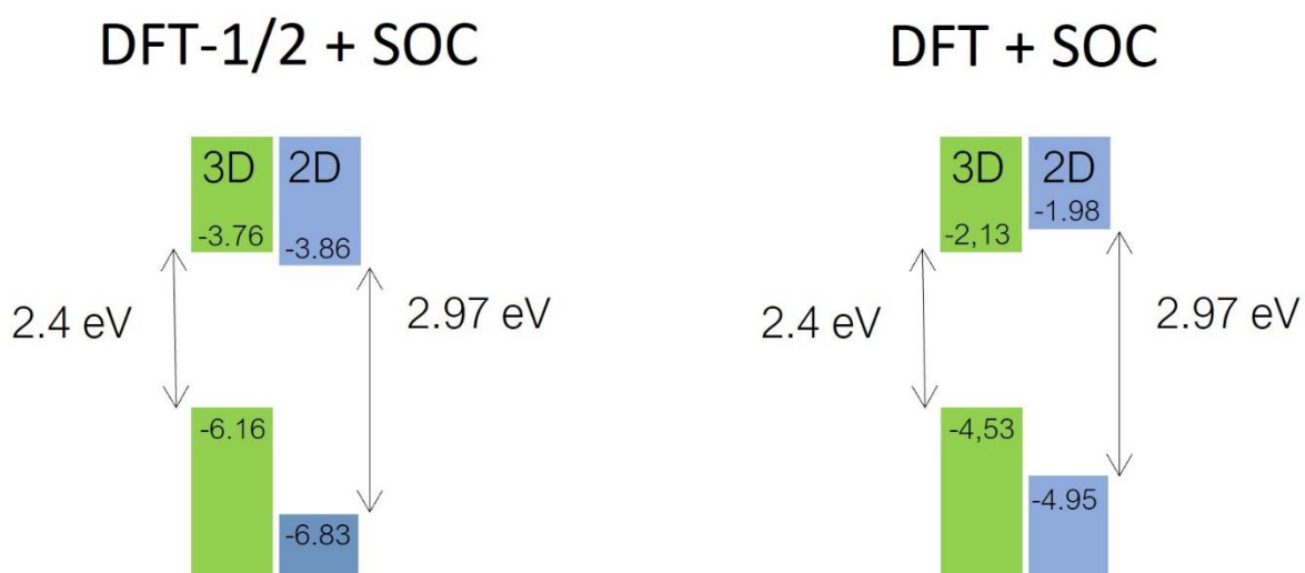
Figure S27 – Plot showing the predicted values of band energy levels of 3D CsPbBr 3 (green) and 2D BA 2 CsPb 2 Br 7 (blue) calculated using single-point calculations with DFT-1/2 (left) and GGA-PBE (right), including spin-orbit coupling, and using experimental optical band gaps.
