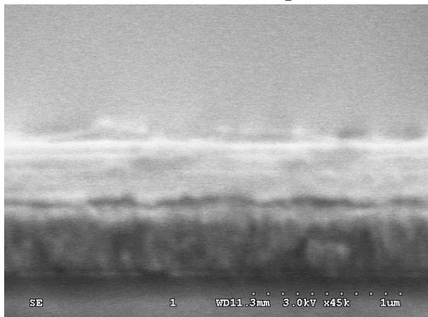
**b) 276 nm ( $\pm 25$  nm) thick perovskite absorber**
