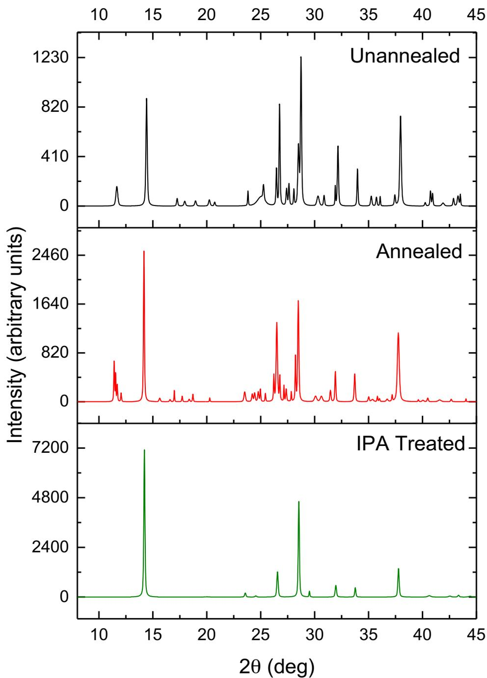
Figure S3: XRD patterns for a MAPbI<sub>3</sub> film fabricated via dual source evaporation<sup>7</sup> on fluorine-doped tin oxide (FTO). A dihydrate (CH<sub>3</sub>NH<sub>3</sub>)<sub>4</sub>PbI<sub>6</sub>·2H<sub>2</sub>O is formed after the bilayer film is exposed to ambient air immediately after the fabrication on the film. After annealing in ambient air, the dihydrate peaks remain. Spin coating IPA on the films clearly shows the removal of the dihydrate and a more crystalline film.
