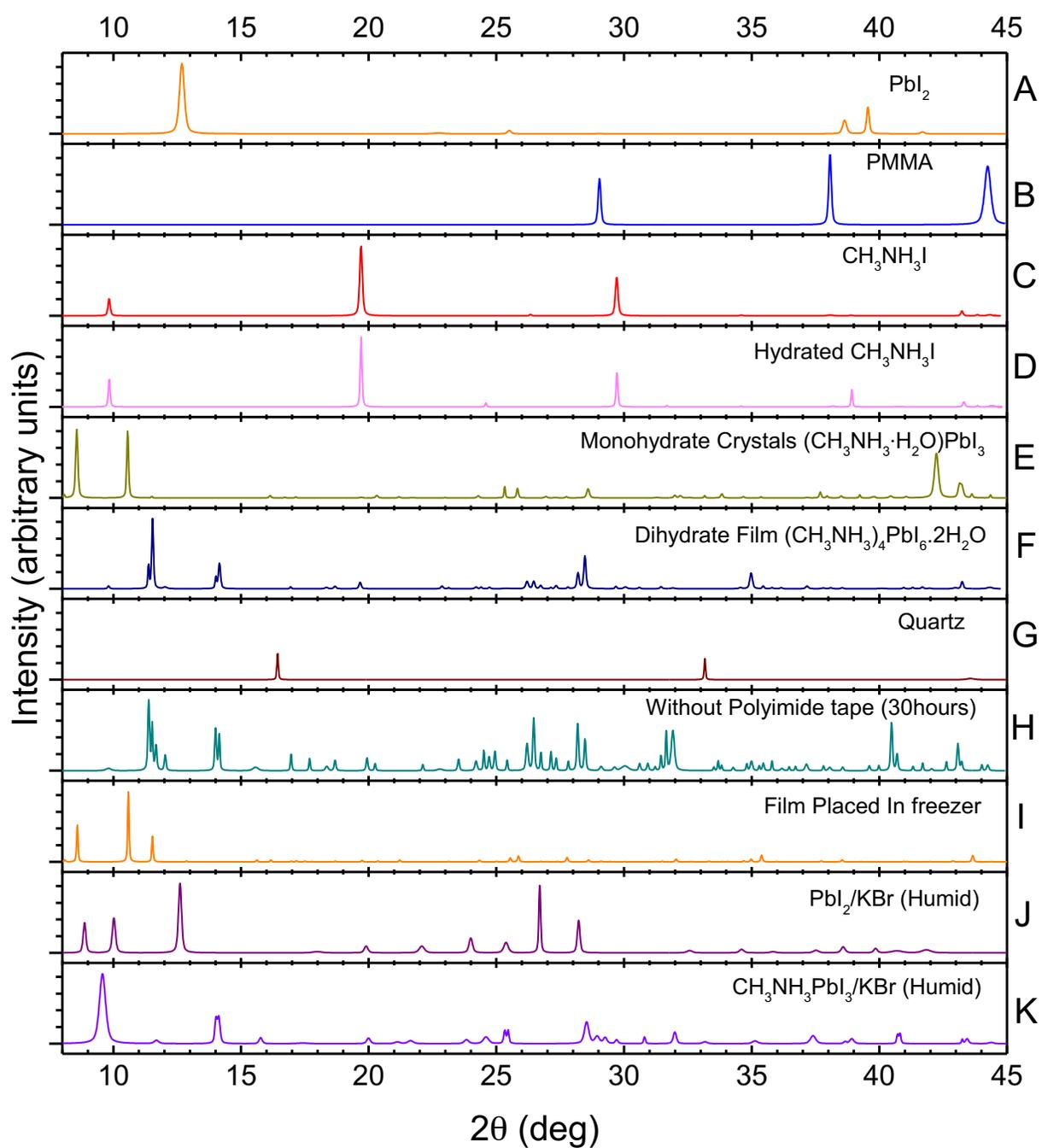
Figure S2. X-Ray diffraction patterns for precursors and derivative compounds associated with intermediates or degradation products of  $MAPbI_3$ . Details about each sample are provided in Table S1.
