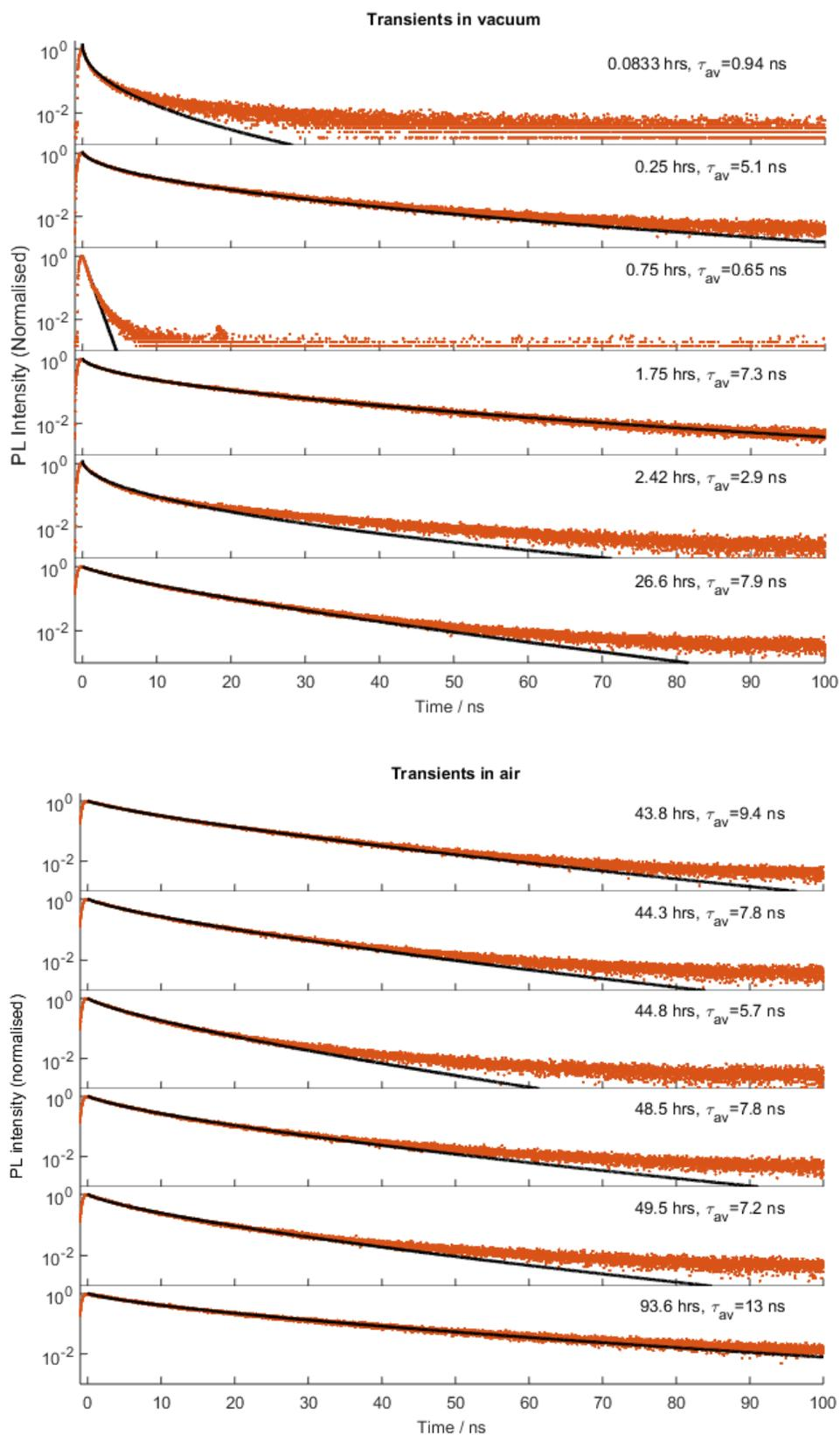
Figure S4. PL transients measured in vacuum and after exposure to ambient air.
