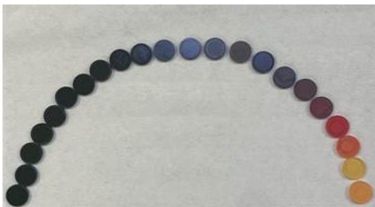
**Figure S1.** Image of  $\text{MAPb}(\text{I}_{1-x}\text{Br}_x)_3$  thin films on z-cut quartz substrates. From left to right, the nominal bromide fraction was: 0, 0.1, 0.15, 0.2, 0.25, 0.3, 0.333, 0.4, 0.425, 0.45, 0.475, 0.5, 0.525, 0.55, 0.575, 0.6, 0.667, 0.7, 0.8, 0.83, 0.9, and 1.
