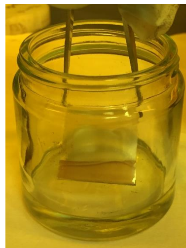
Fig. S3. PAI. Above: Photographs of FASn 0.5 Pb 0.5 I 3 films at different stages of the precursor phase antisolvent immersion deposition technique, showing change in colour of the films. Right: dipping into anisole bath in progress showing change from transparent to reddish colour.
